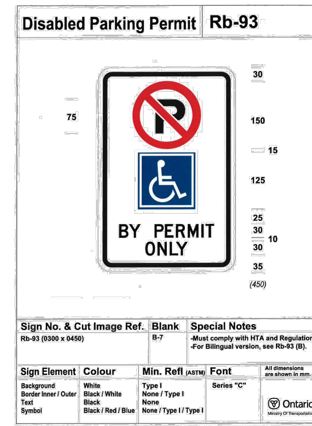
BARRIER FREE PARKING SIGN DETAIL N.T.S.
