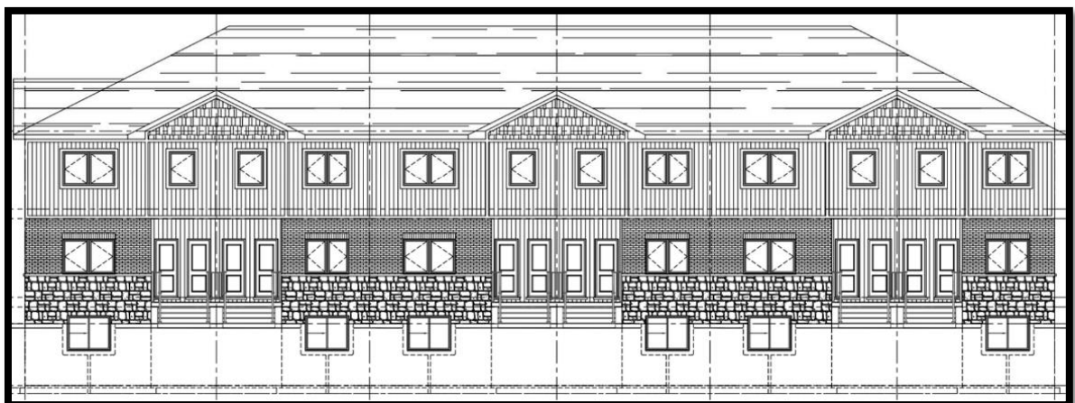
Figure 6 - West-facing elevation drawings of four-unit townhouse block
