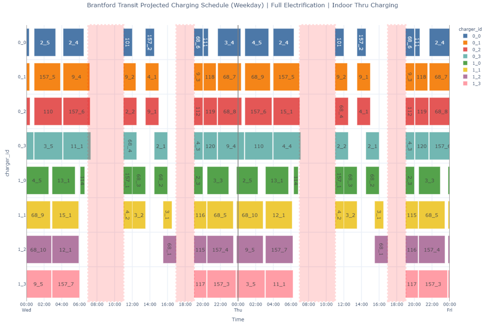
Exhibit 46: Charger schedule (Mon-Sat service, indoor batch charging, 32 BEBs (fully electrified service))
